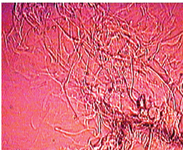
Figure 2 Polarized light microscopy picture of a chitosan solution (DD = 67.2%, M_w = 461 kDa) in 2.96M malic acid ( 10 \times 10 ). [Color figure can be viewed in the online issue, which is available at www.interscience.wiley.com .]
